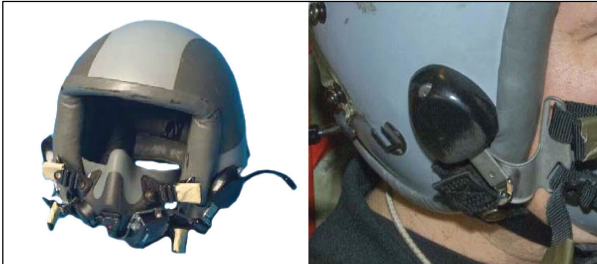
Figure 13-5. Parachutist oxygen mask with bayonet connectors and taped straps
