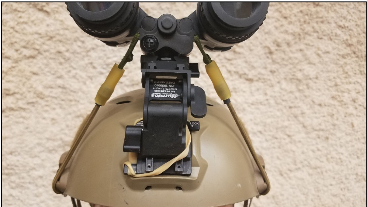
Figure G-2. Latex tubing used to close bungee cord hook fasteners
