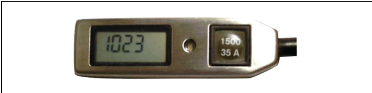
Figure 11-15. Military CYPRES 2 displaying current barometric pressure in millibars
