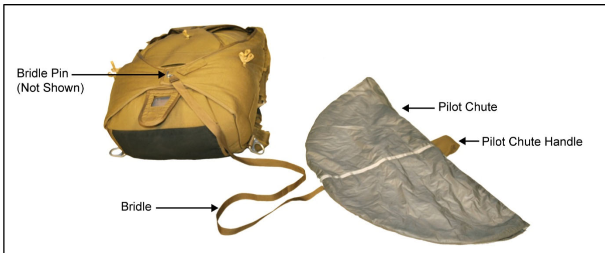
Figure 3-6. Assembly components for military free-fall when jumping in the bottom of container configuration
