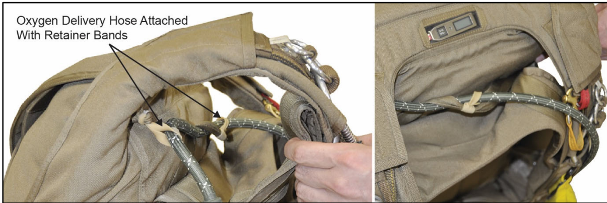
Figure 13-9. Oxygen delivery hose attached
