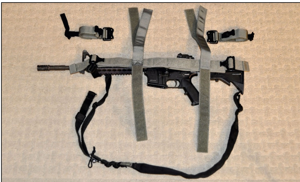
Figure 12-21. Attaching horizontal straps to the pile portion of the weapon harness
