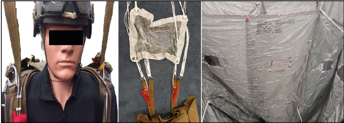
Figure 9-1. Reserve risers and reserve parachute identification during premature activation
