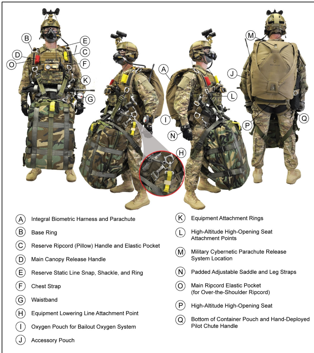
Figure 2-2. RA-1 main components
