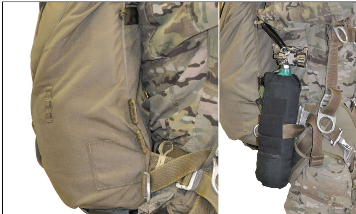
Figure 13-11. A composite 3,000 psi bottle and pouch attached to the jumper
