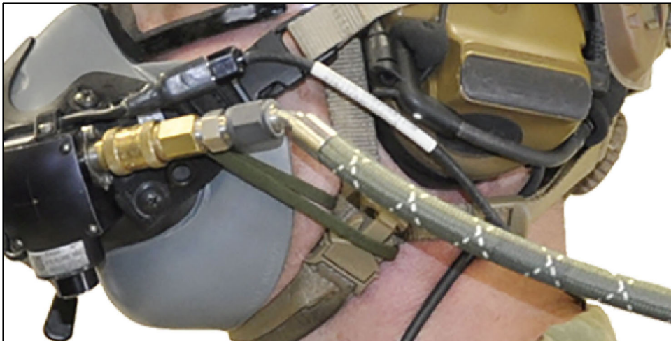
Figure 13-2. Parachutist oxygen mask securing lanyard
