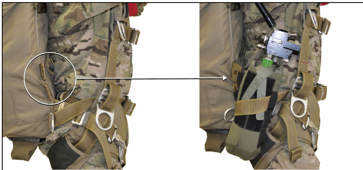
Figure 2-5. Barrel locks attachment point for oxygen system pouch
