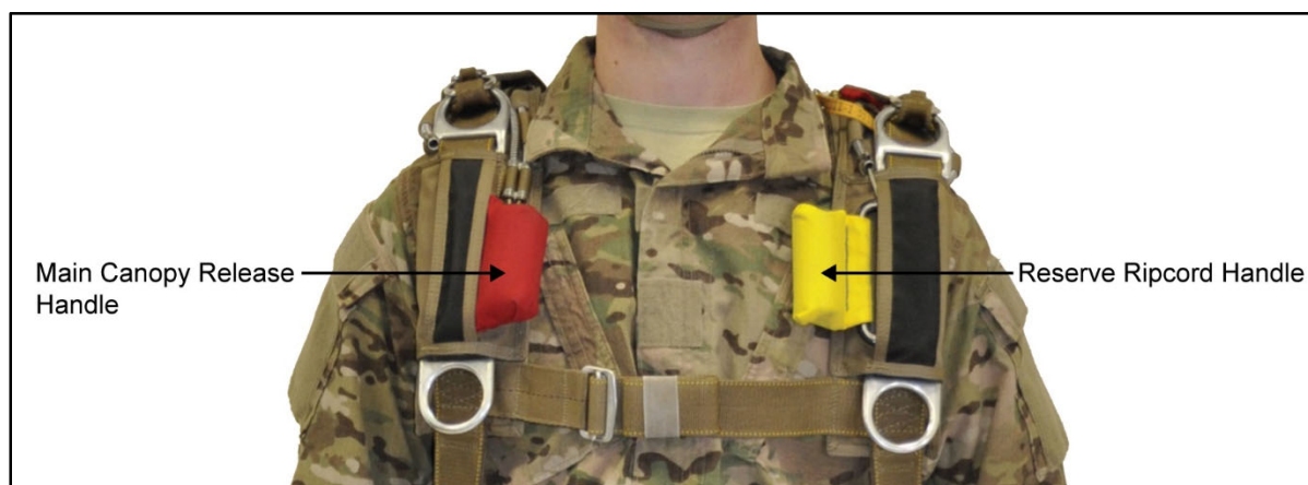
Figure 3-4. Main canopy release handle (red) and reserve ripcord handle (yellow)
