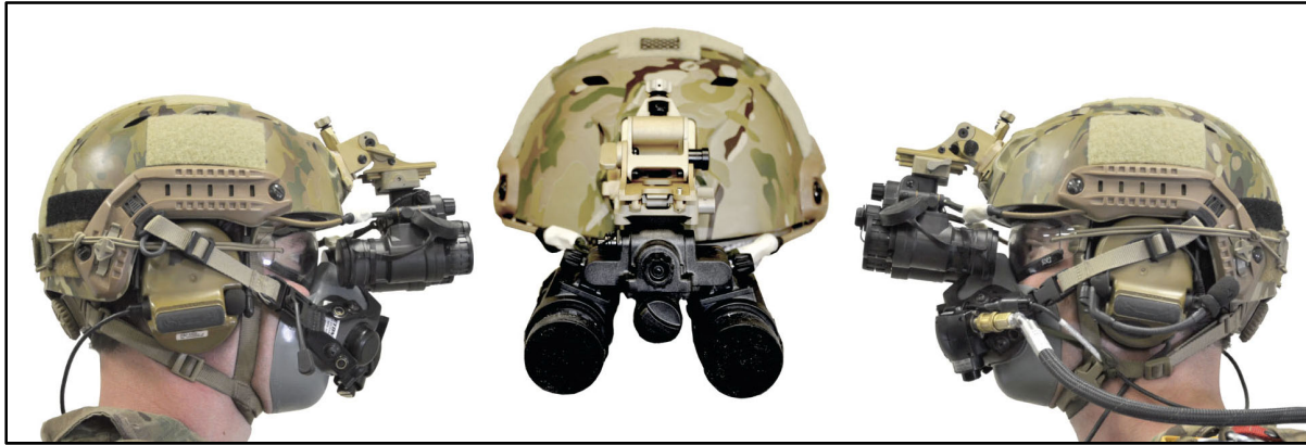
Figure G-3. Bungee position on night vision goggle mount
