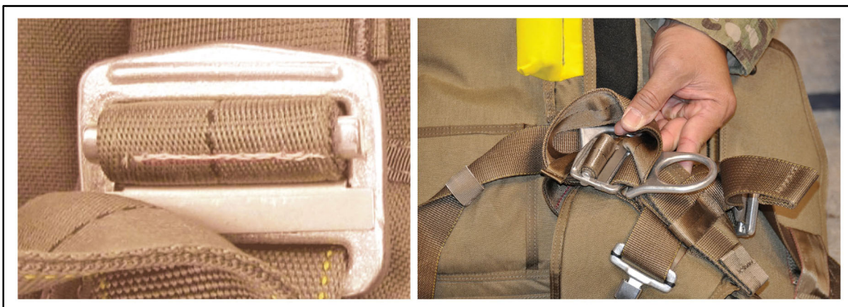
Figure 4-4. Main lift web thread stitching location
