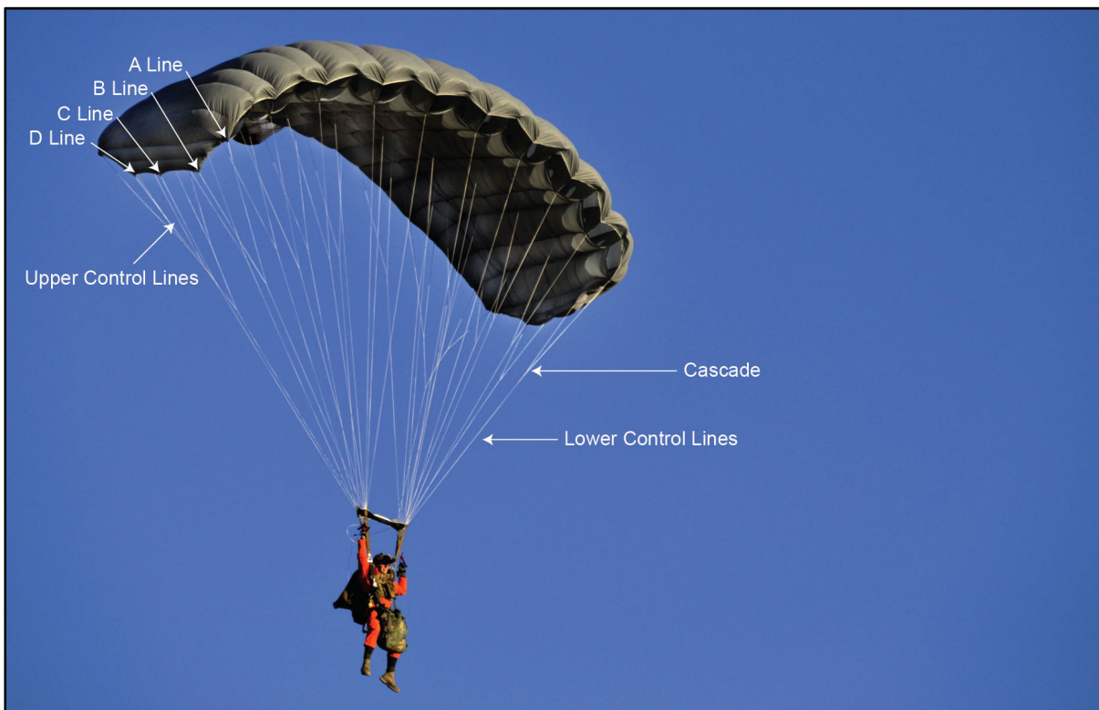
Figure 3-3. Suspension line groups under a deployed canopy
